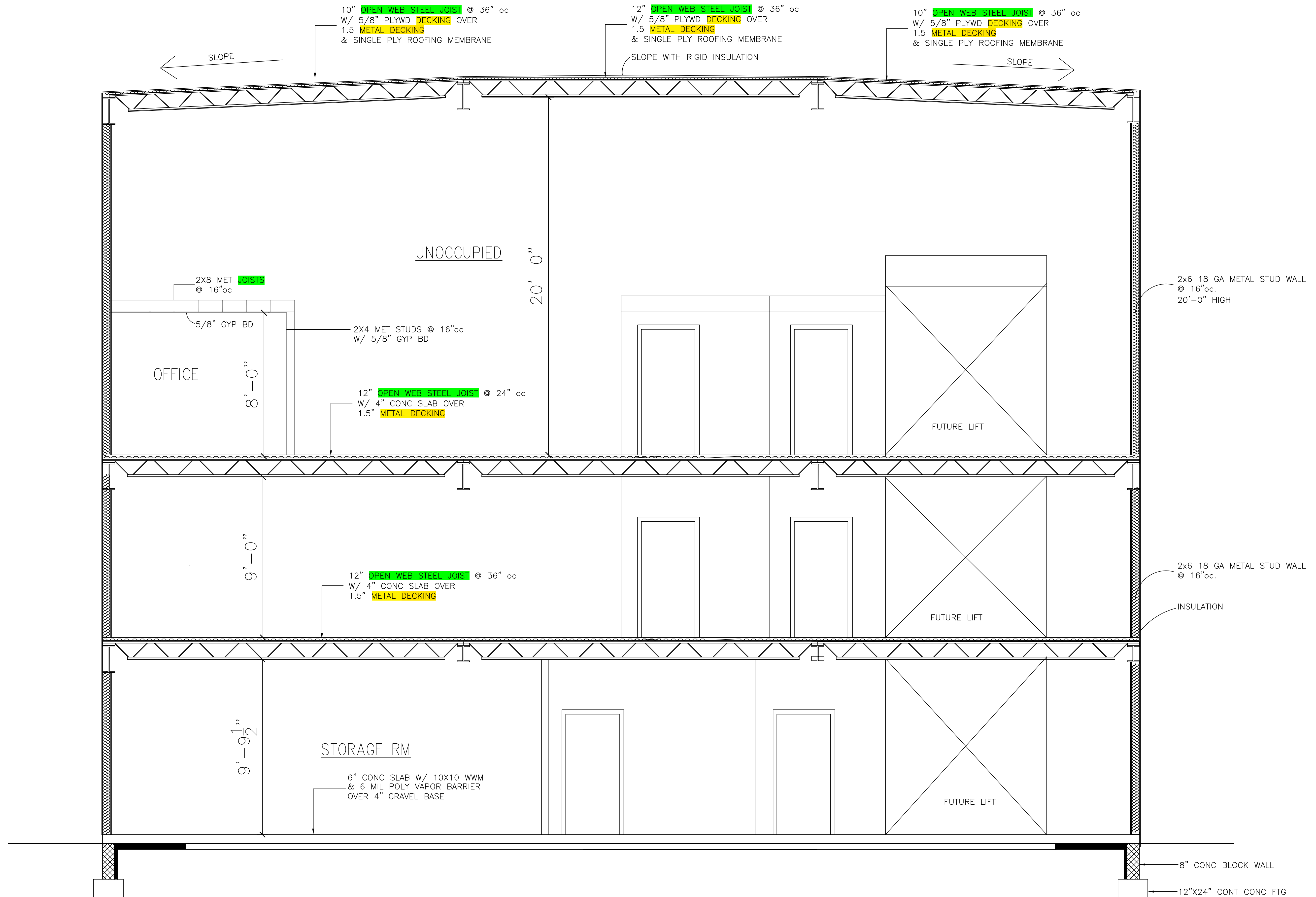
BUILDING SECTION @ MEZZANINE SCALE: 3/8"=1'-0"
