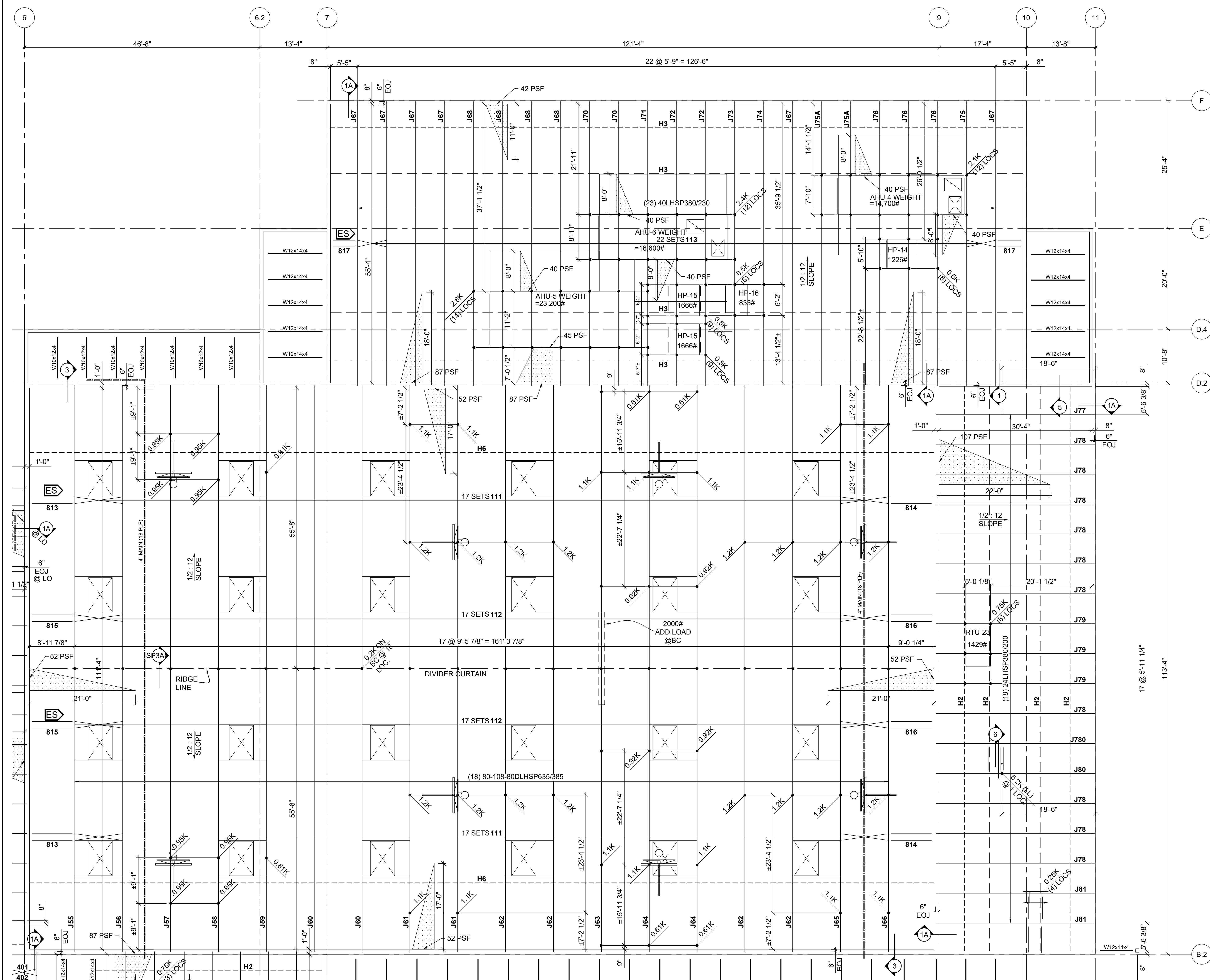
PARTIAL ROOF JOIST PLACEMENT PLAN SEQ. 1 & SEQ. 2 (SPliced JOISTS) REF.: S133
